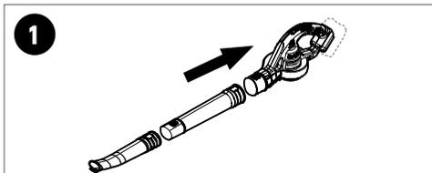
1. Align blower with the upper tube (1), push on to click into place.
