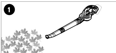
1. Hold blower firmly in hand, slide on/off switch (2) forward.
