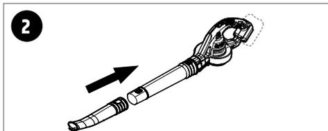
2. Align lower tube (4) with the upper tube, push together to click into place.
