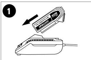
1. ALIGN BATTERY RIBS WITH CHARGER
